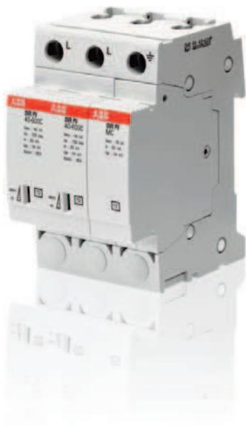
The OVR T2 protects inverters and installations from over voltages and impulse currents, such as switching and lighting surges. The device ensures the limitation of over voltage to an acceptable level for the equipment to be protected.
