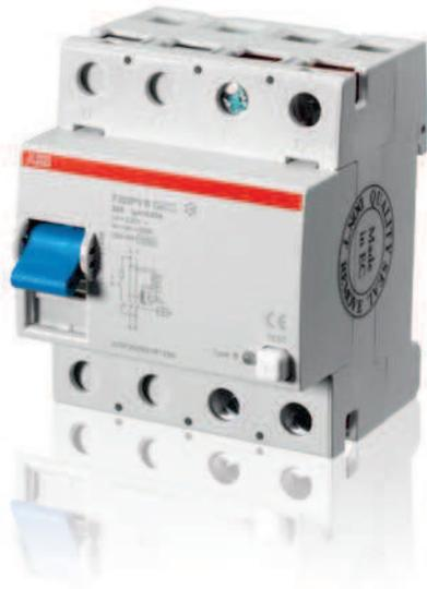
Residual current devices ensure protection of people and installations against fault current to earth and fire risks. An RCD B type is required on the AC side in case of lack of electrical separation between the AC and the DC side.
